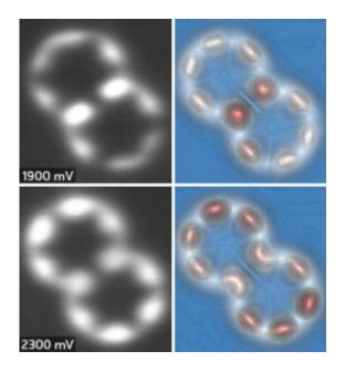
High-resolution microscopy reveals that a benzene-like molecule known as HBC has a quantized electron density around its ring framework (left). Theoretical calculations show that the observed quantum states change with different tip positions (right, upper/lower images, respectively). Credit: 2012 American Chemical Society
