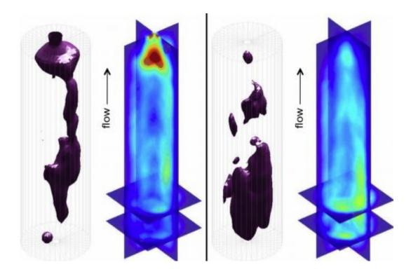
SPECT images of a flow tracer in a sediment column. The left image shows the beginning of the experiment. The right image shows changes six weeks after the start of a test remediation strategy. Early on, the flow was rapid, so most of the tracer is at the flow exit at the top of the column. Later, remediation led to water being retained in regions near the flow inlet (bottom of the column).
