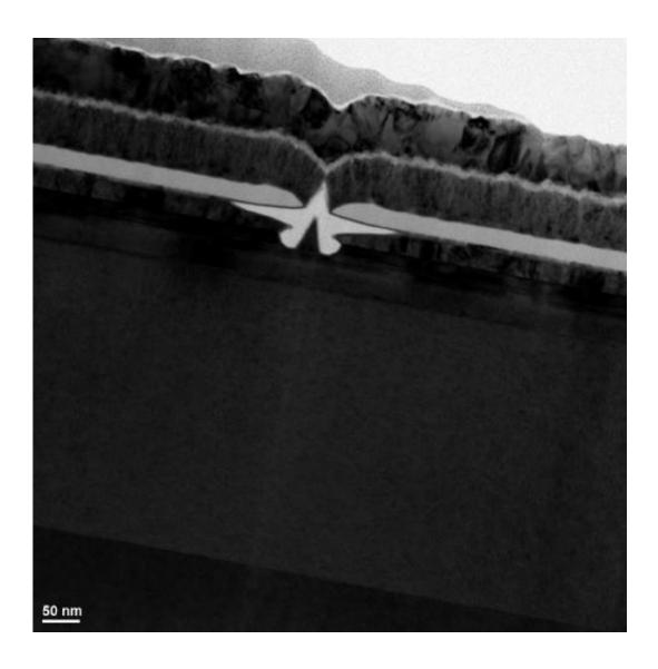
A cross-section transmission electron micrograph of the fabricated transistor. The central inverted V is the gate. The two molybdenum contacts on either side are the source and drain of the transistor. The channel is the indium gallium arsenide light color layer under the source, drain and gate.
