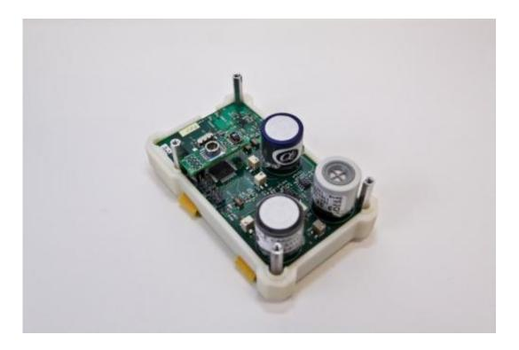
A view of the inside of the CitiSense sensor: the three cylindrical components detect ozone, nitrogen dioxide and carbon monoxide. Credit: Jacobs School of Engineering at UC San Diego
