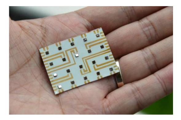
This shows the MEMS underwater MEMS sensor array on the palm of its inventor, Assoc. Prof Miao. Jianmin from Nanyang Technological University. Credit: Nanyang Technological University
