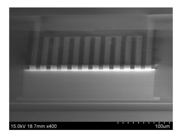
These are experimental images of a self-rolled inductor, printed on a very thin film of silicon nitrate. Credit: Xiuling Li
