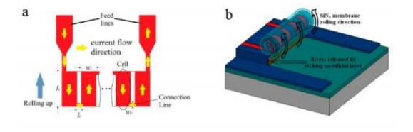
(a) A pattern of conduction strips on a 2D nanomembrane, with arrows indicating the direction of current flow. (b) A nanomembrane rolls up due to stress release. Image credit: Wen Huang, et al. ©2012 American Chemical Society
