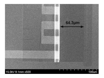
These are experimental images of a self-rolled inductor, printed on a very thin film of silicon nitrate. Credit: Xiuling LI
