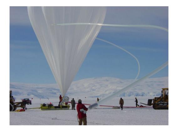
Filling tubes bowing in the wind as TIGER, Super-TIGER's predecessor is prepared for launch in 2003. It takes two trucks of helium to fill a balloon, which will be roughly the size of a football stadium once it ascends to the stratosphere.
