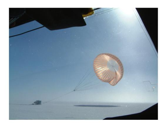
The payload being dragged across the ice after the parachute failed to separate on landing at the end of the first TIGER flight in January 2002. Project engineer John Epstein, since retired, had the presence of mind to snap a photo. Credit: John Epstein
