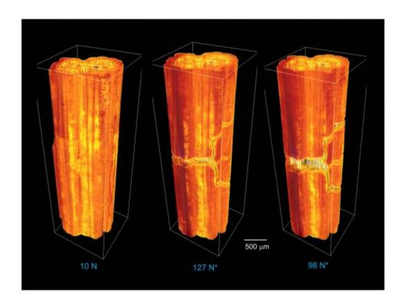
These CT scans showing the formation of microcracks in ceramic composites under applied tensile loads at 1,750 degrees Celsius were obtained at Berkeley Lab's Advanced Light Source through the use of a unique mechanical testing rig. Credit: Robert Ritchie, Berkeley Lab
