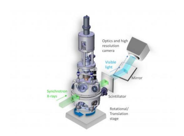
This is a schematic illustration of the in situ ultrahigh temperature tensile test rig for synchrotron X-ray computed microtomography now being used at Beamline 8.3.2 of Berkeley Lab's Advanced Light Source. Credit: Robert Ritchie,
