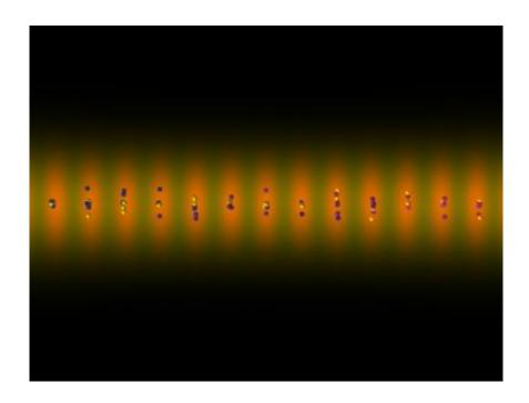
This shows the lattice of laser beams traps small numbers of ytterbium atoms in pancake-shaped "wells." A yellow laser excites the atoms so that they switch between lower (blue) and higher (yellow) energy levels. Credit: NIST
