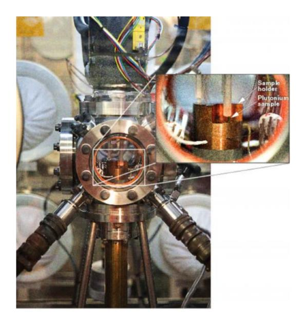
Samples of naturally and artificially aged plutonium, each only 2 or 3 centimeters long, are measured in dilatometry experiments to check for changes in a sample's volume over time.
