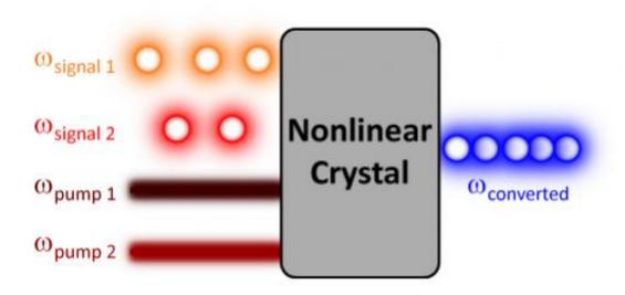
The quantum frequency conversion system uses two pump lasers whose frequency difference is matched to the difference between the two input photon streams, causing the new photons from a nonlinear crystal to be emitted at exactly the same frequency.
