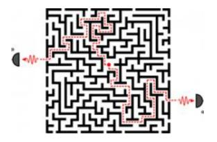
The illustration shows how the scattering of photons occurs in a complex photonic medium. Two photons are emitted from a light source in the centre and move through a labyrinth to illustrate complex scattering. The photons take different paths through the medium, but they are interdependent in the sense that that the chance of observing a photon at one outlet is increased if a photon is observed at the other outlet.
