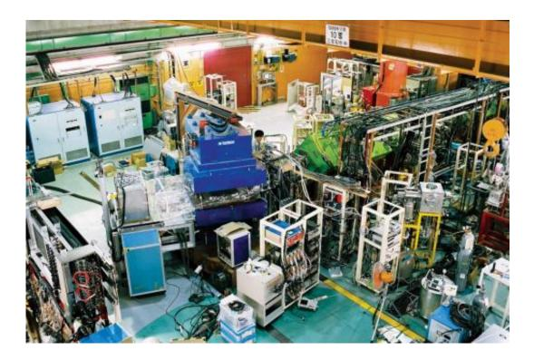
The RIKEN Projectile fragment Separator (RIPS) (pictured) produces highintensity beams of radioactive ions, which help scientists in the study of nuclear processes. Credit: 2012 Yoshiteru Sato, Seoul National University
