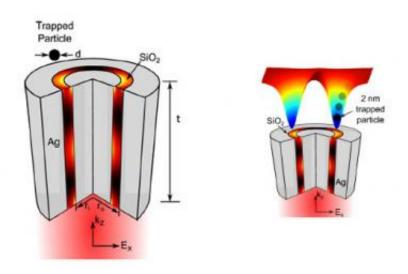
This illustration shows the new aperture design (left) with two layers of silver separated by another of silicon dioxide. The structure focuses light in a novel way to trap particles smaller than ever before. The focused beams are shown in the illustration on the right. Credit: Amr Saleh
