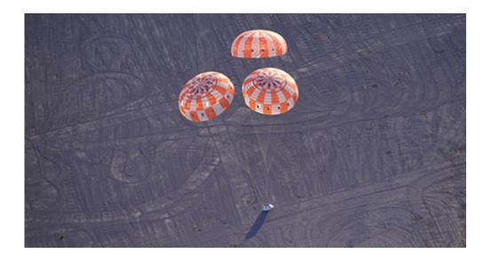
A mockup Orion capsule touches down in the desert of the U.S. Army Yuma Proving Ground in Arizona with the help of its three 300-pound main parachutes, after being dropped from an airplane 25,000 feet up. The test verified that the parachute design for the spacecraft – which will take humans farther than they've ever been before and return them to Earth at greater speeds than ever before – will work in the event of one of the capsule's two drogue parachutes malfunctions. Credit: NASA
