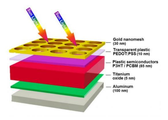
A key part of the new technology is a thin gold mesh, which serves as a "window" layer for the solar cell. Credit: Image courtesy of the Chou lab
