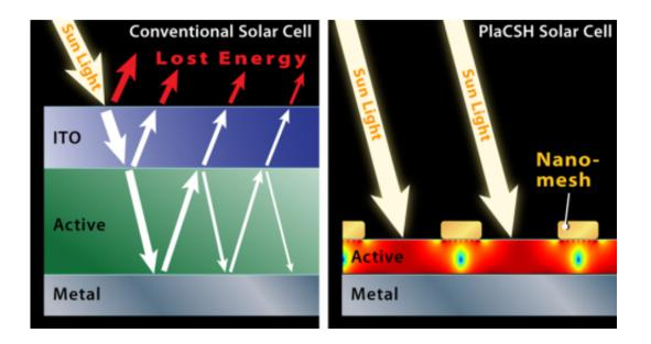
A conventional solar cell, left, reflects light off its surface and loses light that penetrates the cell. New technology, right, develop by Princeton professor Stephen Chou and colleagues in electrical engineering, prevents both types of loss and is much thinner. Credit: Illustration by Dimitri Karetnikov
