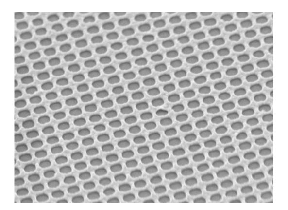
This electron microscope image shows the gold mesh created by Chou and colleagues. Each hole is 175 nanometers in diameter, which is smaller than the wavelength of light. Credit: Image courtesy of the Chou lab
