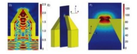
Electromagnetic fields are enhanced in the gap as the campanile squeezes light beyond the diffraction limit, as shown in these simulations. Credit: Lawrence Berkeley National Lab
