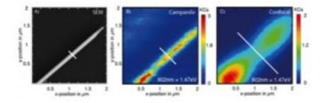
Using the campanile tip, Berkeley Lab researchers take "color" images with nanoscale resolution. A photovoltaic indium-phosphide nanowire is easy to see in a black-and-white electron micrograph (left) but chemical information has low resolution in a normal confocal micrograph (right). The campanile tip reveals both shape and chemistry of a nanowire (center). Credit: Lawrence Berkeley National Lab
