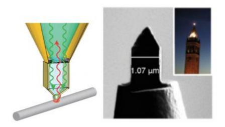
A new microscopy tool promises to revolutionize nanoscale imaging. Left, a design schematic of the so-called "campanile" microscopy tip. Right, an electron micrograph of the tip and, inset, the UC Berkeley campanile bell-tower for which it is named. Credit: Lawrence Berkeley National Lab
