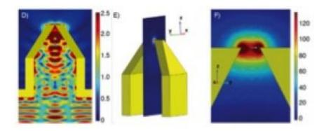
Electromagnetic fields are enhanced in the gap as the campanile squeezes light beyond the diffraction limit, as shown in these simulations. Credit: Lawrence Berkeley National Lab
