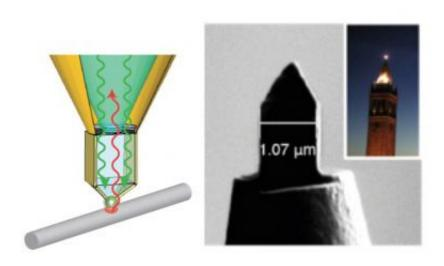
A new microscopy tool promises to revolutionize nanoscale imaging. Left, a design schematic of the so-called "campanile" microscopy tip. Right, an electron micrograph of the tip and, inset, the UC Berkeley campanile bell-tower for which it is named. Credit: Lawrence Berkeley National Lab
