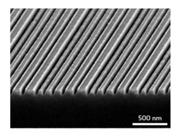
A scanning-electron micrograph of a test sample used to demonstrate a superlens's resolving power of better than 50 nanometers. Credit: 2012 A\*STAR Institute of Materials Research and Engineering
