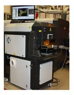
The state-of-the-art ultraviolet laser that will be used with EMSL's new laser ablation capillary absorption instrument.
