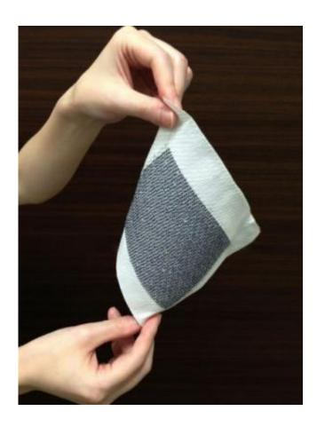
Image provided by Sphelar Power on December 11 shows small spherical solar cells woven into a piece of fabric. The new fabric is made of wafer-thin solar cells woven together that could see people powering up their electronics with their sweater or trousers.
