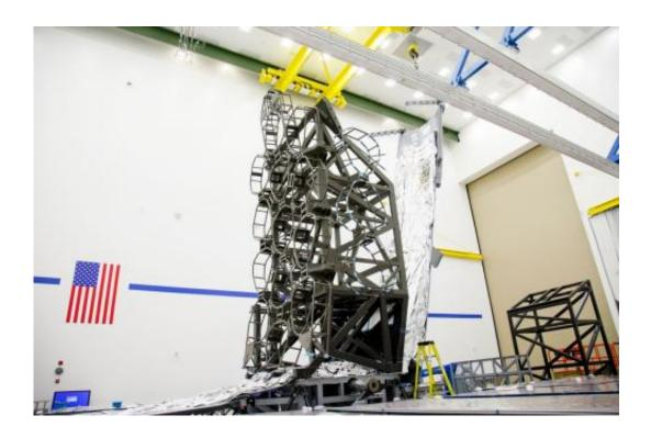
Engineers at Northrop Grumman Aerospace Systems in Redondo Beach, Calif. installed the first of five template sunshield membranes on a Webb telescope mock-up. The mock-up is a full-scale structural facsimile of the real observatory. Credit: Northrop Grumman
