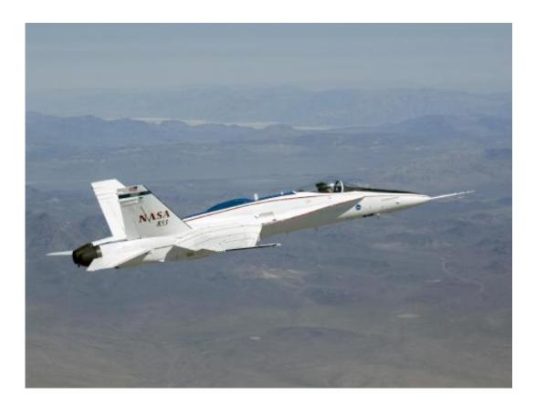
NASA Dryden's versatile F/A-18A Full Scale Advanced Systems Testbed (FAST) aircraft recently completed flying the Intelligent Control for Performance (ICP) research project that explored reducing fuel consumption during cruise flight by modifying control laws and mechanisms in the aircraft's flight control computer. Credit: NASA/Lori Losey
