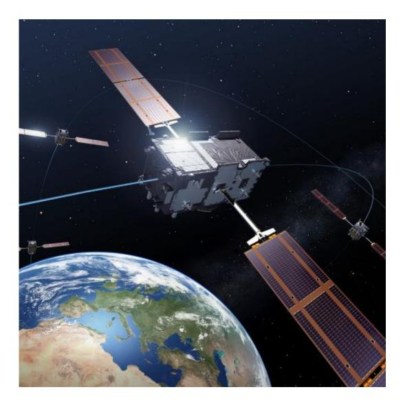
Four Galileo In-Orbit Validation satellites in medium-Earth orbit, the minimum number needed to perform a navigation fix. Credit: ESA – P. Carril
