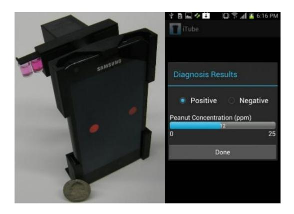
Left: The iTube platform, which utilizes colorimetric assays and a smart phone-based digital reader. Right: A screen capture of the iTube App.
