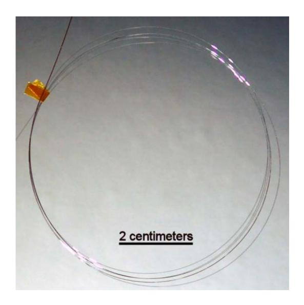
A coiled strand of a meter-long solar-cell junction fiber, thinner than the width of a human hair, which has been created by a team of chemists, physicists, and engineers led by John Badding at Penn State University. Credit: Badding lab, Penn State University
