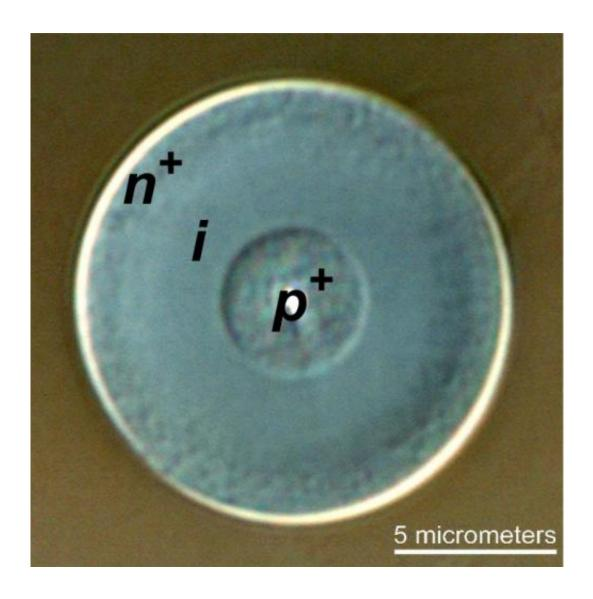
A cross-sectional image of the new silicon-based optical fiber with solar-cell capabilities. Shown are the layers -- labeled n+, i, and p+ -- that have been deposited inside the pore of the fiber. Credit: Badding lab, Penn State University
