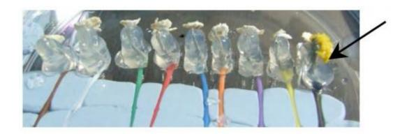
Photo of an example setup. The reference electrode is on the right side. The other 8 electrodes are measurement electrodes. They are covered with blobs of non-nutrient agar and oat flakes placed on top of each. At the beginning, a piece of plasmodium is placed on top of agar blob covering the reference electrode only (indicated by the dashed circle). Credit: arXiv:1212.1203 [nlin.PS]
