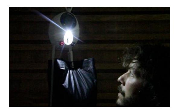
(Phys.org)—London based designers Martin Riddiford and Jim Reeves have created what they are calling the GravityLight, an LED lamp that runs off of nothing but gravity. The purpose of the lamp is to provide people in third world countries with an alternative to kerosene lamps which cause burns and lung ailments to millions of people too poor to afford any other source of light.
