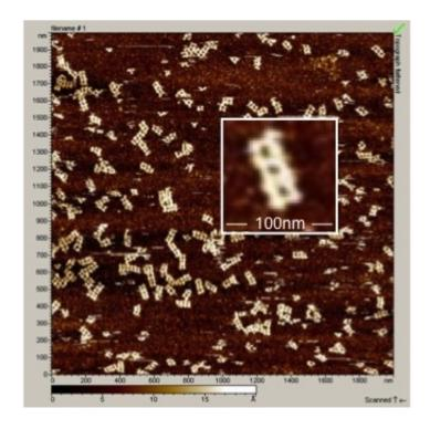
A collection of pharmaceutical molecules is shown after self-assembly. The detail shows a single molecule, made up of strands of DNA, a therapeutic agent and other components that improve its ability to target cancer. Credit: Parabon NanoLabs
