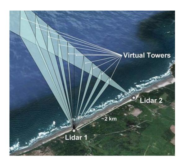
Conceptual drawing of proposed dual Doppler lidar scanning technique installed on the coastline. The two Doppler lidars are installed approximately two kilometers apart and set up to scan the same area of the atmosphere. Data will be combined to provide measurements of the detailed wind field in the regions where the scans overlap or intersect (virtual towers).
