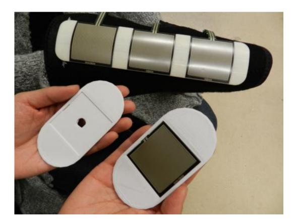
The current prototype of the Access4Kids device (top right) includes three forcesensitive resistors that measure pressure and convert it into a signal that instructs the tablet. Howard is creating a second prototype with wireless sensors (bottom left) that can be placed anywhere a child is capable of hitting them.
