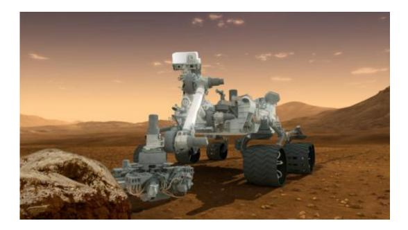
This artist's concept features NASA's Mars Science Laboratory Curiosity rover, a mobile robot for investigating Mars' past or present ability to sustain microbial life. Credit: Credit: NASA/JPL-Caltech
