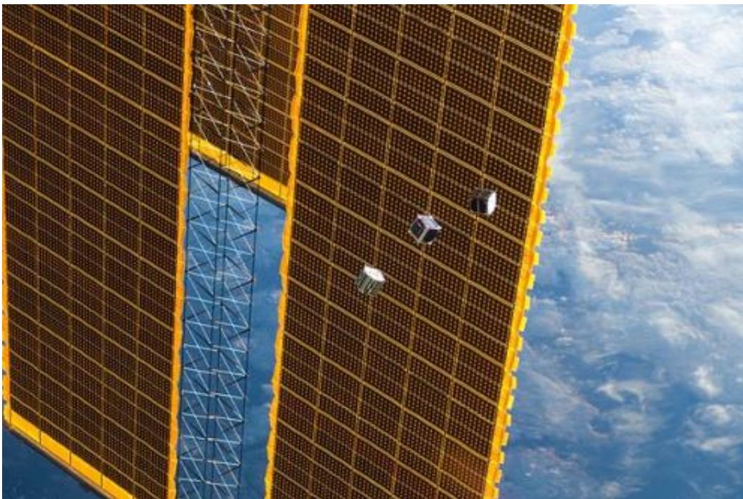
FITSAT-1, F-1, and TechEdSat Cube Satellites after deployment from the International Space Station. Credit: NASA
