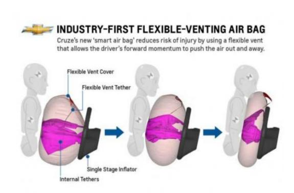
The 2013 Chevrolet Cruze introduces an industry-first driver-side air bag that uses a flexible venting technology designed to deploy more efficiently while providing equivalent crash protection to more expensive and complex air bag systems.
