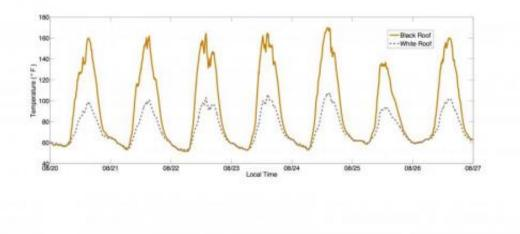
Temperature Chart: This chart shows the temperature fluctuations on a white roof compared to a black roof at PPPL during the last week of August. The black roof reached 170 degrees Fahrenheit, while the top temperature of the white roof was just over 100 degrees.
