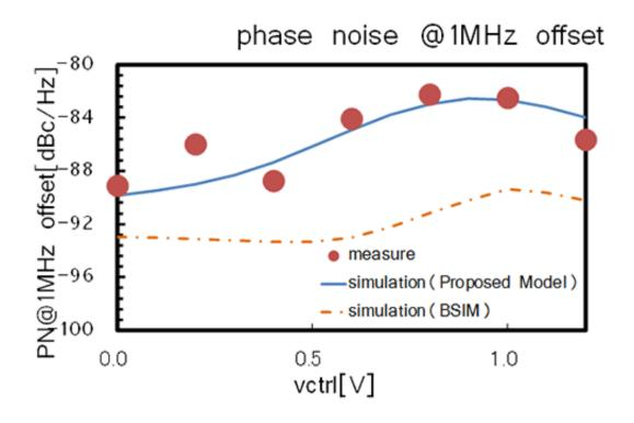
Toshiba Corporation today announced the development of a compact MOS-Varactor simulation model that delivers high level accuracy from DC to the millimeter wave (60 GHz) region. The new model was developed in cooperation with Professor Nobuyuki Itoh of Okayama
