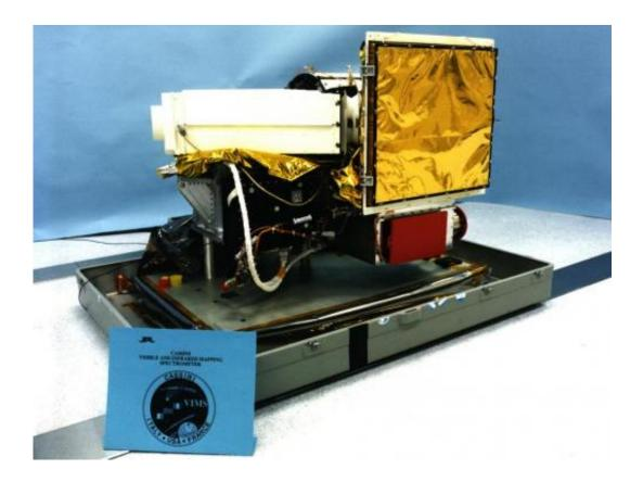
This image shows the visual and infrared mapping spectrometer instrument just before it was attached to NASA's Cassini spacecraft. Image credit: NASA/JPL-Caltech/University of Arizona
