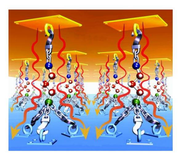
A team of interdisciplinary researchers at Rensselaer Polytechnic Institute has developed a new method for significantly increasing the heat transfer rate across two different materials. By sandwiching a layer of ultrathin [2]nanoglue[2] between copper and silica, the research team demonstrated a four-fold increase in thermal conductance at the interface between the two materials. Credit: Rensselaer/Ramanath
