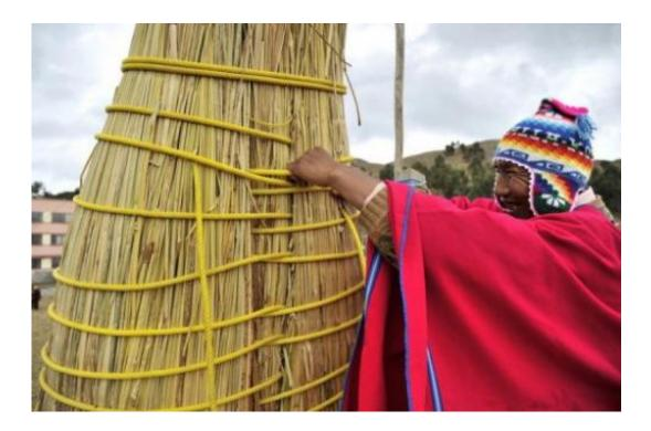
A man works on the construction of a reed boat or "Thunupa" on Suriqui island in Lake Titicaca, Bolivia, on December 2, 2012. Ships built of bullrush reed have sailed the Pacific, the Atlantic, the Mediterranean, and for a millennia across the Titicaca, the vast Andean lake 4,700 meters (15,420 feet) above the sea level shared by Bolivia and Peru.
