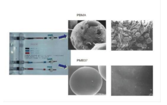
Microsphere columns after passage of whole blood for 15 min (left) and scanning electron microscopy images of polymer-coated beads packed in the columns (right). Credit: Sci. Technol. Adv. Mater. Vol 13 (2012) p. 064101
