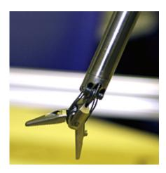
Close-up of one of the RAVEN robot's two pincers, which can hold a needle for simulated suturing.
