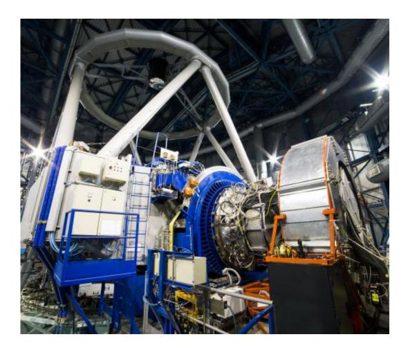
The KMOS instrument mounted on ESO's Very Large Telescope at the Paranal Observatory in Chile. KMOS is unique as it will be able to observe not just one, but 24 objects at the same time in infrared light and to map out how their properties vary from place to place. It will provide crucial data to help understand how galaxies grew and evolved in the early Universe -- and provide it much faster than has been possible up to now. KMOS was built by a consortium
