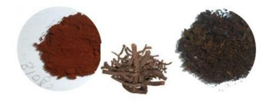
Purpurin, left, extracted from madder root, center, is chemically lithiated, right, for use as an organic cathode in batteries. The material was developed as a less expensive, easier-to-recycle alternative to cobalt oxide cathodes now used in lithium-ion batteries. Credit: Ajayan Lab/Rice University
