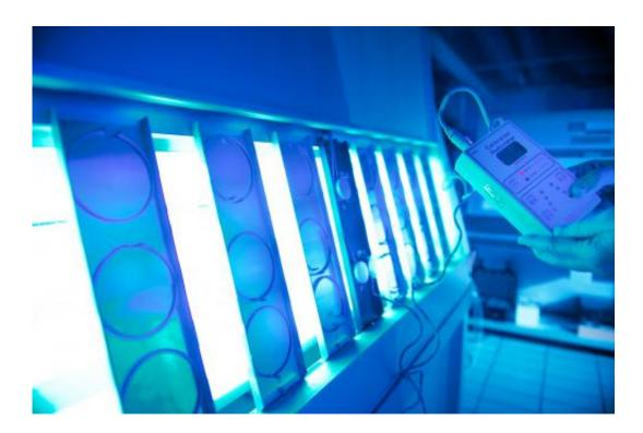
This shows the calibration of the teststand for coatings. Credit: Wolfram Scheible/Fraunhofer
