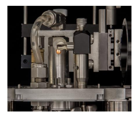
The jet-target area shown in partially disassembled apparatus. The tube at left feeds the water reservoir above the vacuum chamber. Credit: Jens Uhlig
