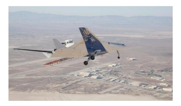
The upgraded X-48C version of Boeing's Blending Wing Body subscale research aircraft banks over Rogers Dry Lake near "Contractors' Row" at Edwards Air Force Base during a test flight Oct. 16, 2012. Combined with the earlier X-48B version, the X-48 technology demonstrator has now flown 100 test missions, more than any other single unmanned X-plane. Credit: NASA/Carla Thomas
