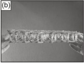
A model of two-dimensional glass: Measurements made by the Max Planck researchers in Berlin prove that disordered silica forms a structure in which not only hexagonal shapes, but also pentagonal and heptagonal ones are often created. The more the ring size deviates from the hexagon, which is the only
