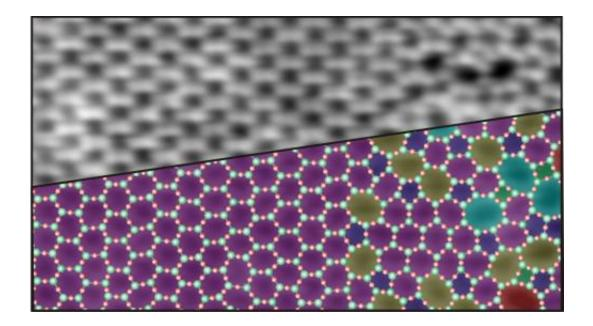
The order disintegrates: During the transition from a crystalline to an amorphous silica structure, rings with five and seven atoms appear first, elements with a larger deviation from the hexagonal rings of the crystalline structure can be found only deeper in the disordered region. Credit: Markus Heyde/Fritz Haber Institute of the MPG
