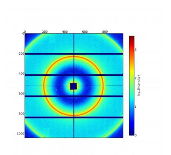
Small-angle X-ray scattering of a micro-vesicle sample (multilamellar liposomes) using the vacuum-compatible Pilatus detector, image recorded at a photon energy of 3 keV. The scattering pattern allows the dimensions of the nano-objects in the examined sample to be determined. Credit: PTB
