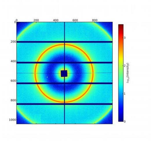
Small-angle X-ray scattering of a micro-vesicle sample (multilamellar liposomes) using the vacuum-compatible Pilatus detector, image recorded at a photon energy of 3 keV. The scattering pattern allows the dimensions of the nano-objects in the examined sample to be determined. Credit: PTB
