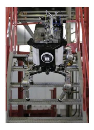
Toshiba Corp.'s nuclear Inspection robot climbs stairs during a demonstration at a Toshiba factory in Yokohama, west of Tokyo, Wednesday, Nov. 21, 2012. The four-legged robot is designed to help at the meltdown-crippled Japanese nuclear plant, climbing over debris and venturing into radiated areas off-limits to human workers. (AP Photo/Itsuo Inouye)
