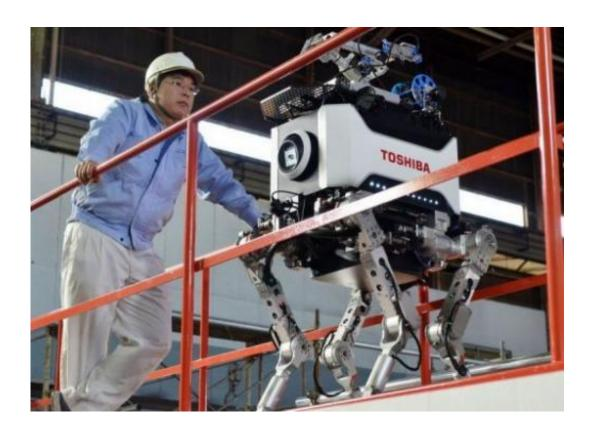
Engineers inspect Toshiba's four-legged robot during a demonstration at Toshiba's technical center in Yokohama, suburban Tokyo. The tetrapod, which weighs 65 kilograms (143 pounds) and is about one metre (3 foot, four inches) tall, is designed to be able to cover difficult terrain—such as going up steep steps—that regular robots struggle with.
