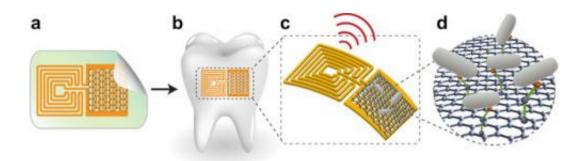
The sensor (A), attached to a tooth (B) and activated by radio signals (C), binds with certain bacteria (D). Credit: Manu Mannoor/Nature Communications
