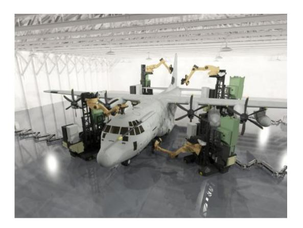
This rendering shows how several robots might be deployed to strip coatings from a C-130 cargo plane. Credit: National Robotics Engineering Center
